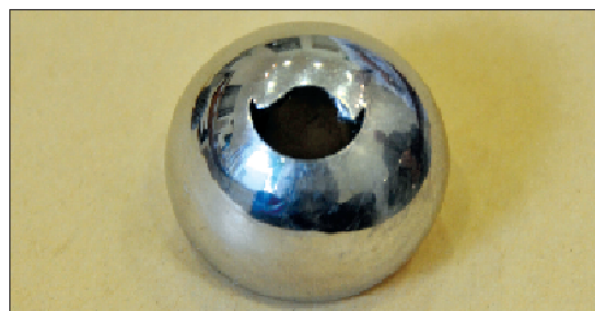
Figure 1. Metal hip prosthesis causing cobalt intoxication. Removed metal head with hole due to severe metal loss.
